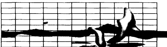
Figure 16 (a) Contour surface of low-pressure and low-speed regions in Case 0 ( \alpha = 0 ): gray, p'^+ < -4.0 ; black, u'^+ < -4.0 ; (b) contour surface of low-pressure and low-speed regions in Case 1C ( \alpha = 4 at 0 < y^+ < 20 ): gray, p'^+ < -4.0 ; black, u'^+ < -4.0
