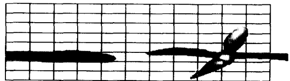
Figure 16 (a) Contour surface of low-pressure and low-speed regions in Case 0 ( \alpha = 0 ): gray, p'^+ < -4.0 ; black, u'^+ < -4.0 ; (b) contour surface of low-pressure and low-speed regions in Case 1C ( \alpha = 4 at 0 < y^+ < 20 ): gray, p'^+ < -4.0 ; black, u'^+ < -4.0
